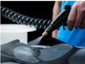
Press the spray gun and wet the electrodes; pump stops after the spraying is finished
